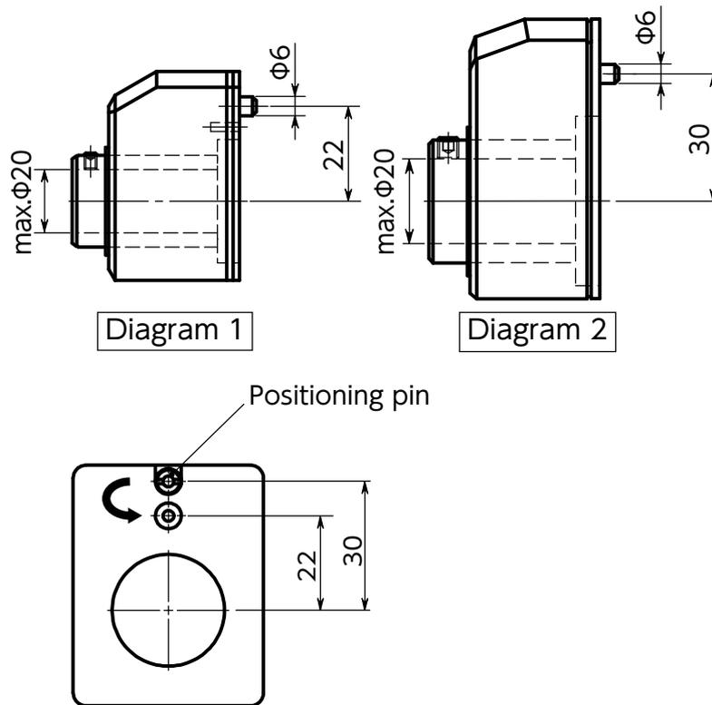
1. **Mount by aligning the unit's positioning pins with the adapter plate mounting holes.**
