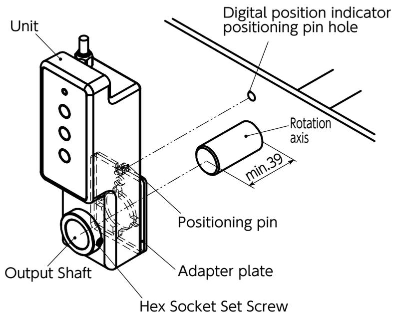
**■ If installing the unit using a collar (optional)**
