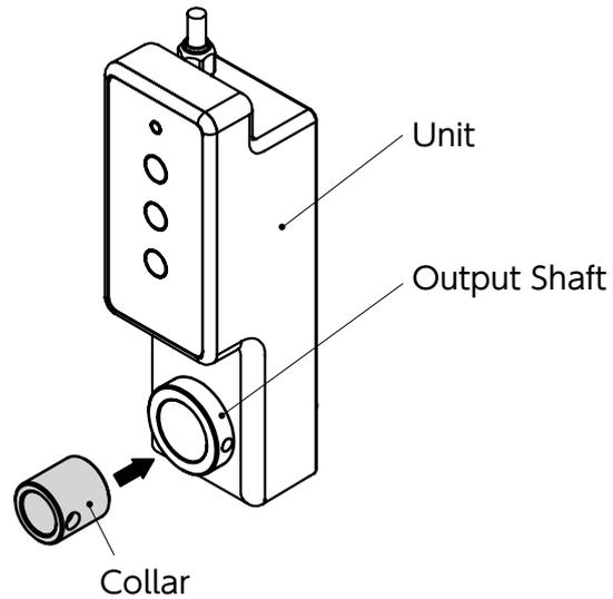
2. Align the unit's output shaft screw holes with the collar's screw through-holes, then mount using the hex socket set screws supplied with the collar.
