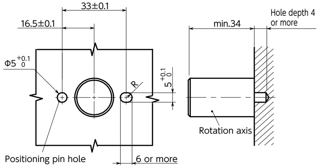
\*Make one of the two positioning pin holes into a slot as per the figure. If machining a slot is difficult, drill out a  $\Phi 6$  or larger round hole.
