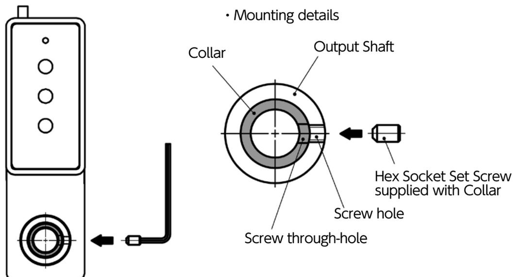
3. With the collar mounted, pass the rotation axis over the unit's output shaft and secure with a hex socket set screw. (Recommended tightening torque: 2.8 N·m)
