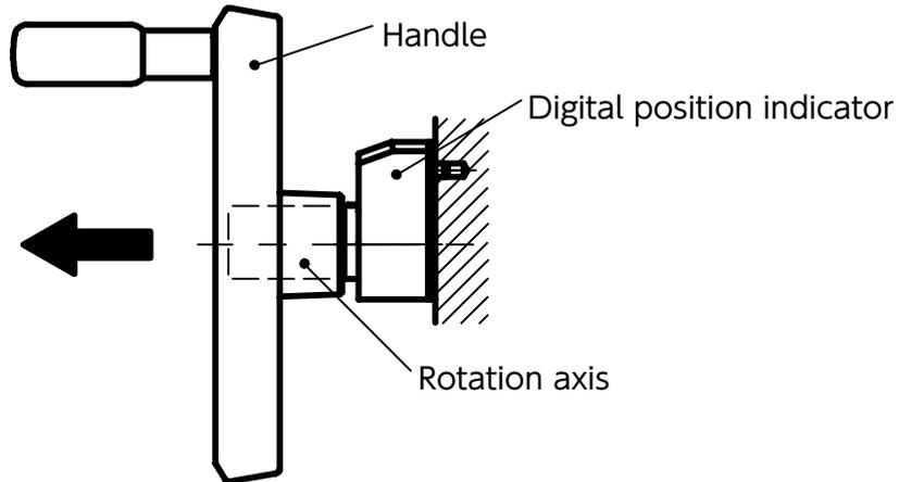
3. With the unit mounted to the adapter plate, pass the rotation axis over the output shaft and secure with the hex socket set screws supplied with the unit. (Recommended tightening torque: 2.8 N·m)
