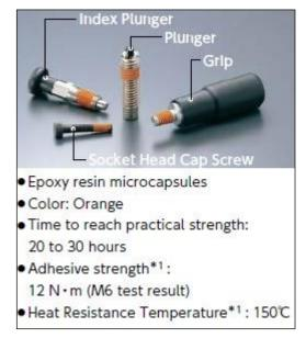
\*1: The adhesion force is the result of M6 testing. It also indicates the loosening torque when tightened at 8 N·m. The heat resistant temperature indicates the limit temperature at which the loosening torque exceeds the tightening torque. The above values are for reference only. They are not guaranteed values. Make sure that there is no problem with your final product when using them.
