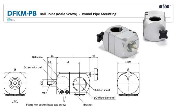
Material/Finish ♠ RoHS **DFKM-PB** A6063 Ball Case Anodized S45C Screw with ball Trivalent Chromate Treatment Fixing Hex Socket Head Cap Screw SCM435 (M5×16mm) Ferrosoferric Oxide Film A6063 Bracket Anodized Rubber sheet NR (Natural Rubber)
