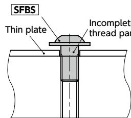
Thin plate fixing socket button head cap screw with flange
