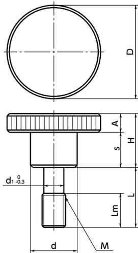
• To distinguish **KNMS-SC** (SUS304) from **KNML-SC** (SUS316L equivalent), **KNML-SC** has a groove on its seating surface.
