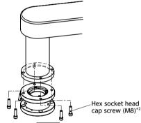
With the **DKSF** locating disk facing downward, fix **DKSF** to the equipment with 4 hex socket head cap screws (M8)\*2.
