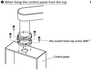
Fix the control panel with 4 hex socket head cap screws (M8)\*2.
