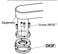
With the **DKSF** locating disk facing downward, fix **DKSF** to the equipment with 4 screws (M10)\*2.
