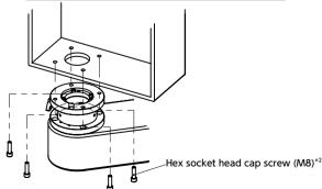
Fix the control panel with 4 hex socket head cap screws (M8)\*2.
