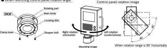
The control panel rotation angle can be restricted through a combination of the mounting position of the provided stopper bolts and the position of the locating disk.
