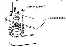
Fix the control panel with 4 screws (M10)\*2.
