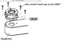
With the **DKSF** locating disk facing downward, fix **DKSF** to the equipment with 4 hex socket head cap screws (M8)\*2.
