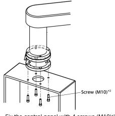
Fix the control panel with 4 screws (M10)\*2.
