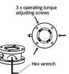
To increase the operating torque, adjust by tightening the 3 operating torque adjusting screws equally.
