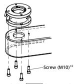
With the **DKSF** locating disk facing downward, fix **DKSF** with 4 screws (M10)\*2.
