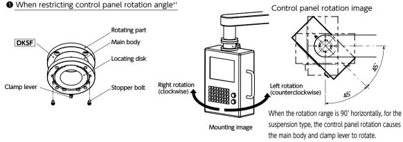
The control panel rotation angle can be restricted through a combination of the mounting position of the provided stopper bolts and the position of the locating disk.
