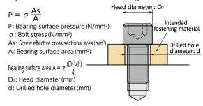
• Head Diameter and Screw Effective Cross-Sectional Area
