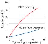
• Reference data for Hex Socket Head Cap Screw - SUSXM7 - PTFE Coating SNSS-M5-25-TF.
