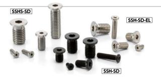
Socket head cap screws with special low profiles and small head diameters. This makes it possible to reduce the spot facing diameter compared to standard socket head cap screws with special low profiles.
