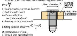
• Head Diameter and Screw Effective Cross-sectional Area
