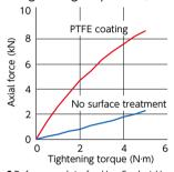
• Reference data for Hex Socket Head Cap Screw - SUSXM7 - PTFE Coating SNSS-M5-25-TF.
