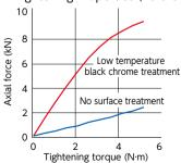
• Reference data for Hex Socket Head Cap Screw - SUSXM7 - Low Temperature Black Chrome Treatment SNSS-M5-25-RY.
